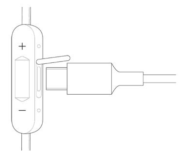
When Flyer is charging, the LED changes color depending on the current charge level. Your headphones are fully charged when the LED is white. Charging fully may take up to 2 hours. For information on what the color of the LED represents while Flyer is charging, see the table below.
