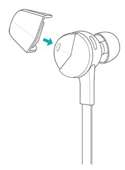
To remove a wing or fin, pinch the base of it between your fingers and pull away from the earbud to slide it out of the rounded slot.
